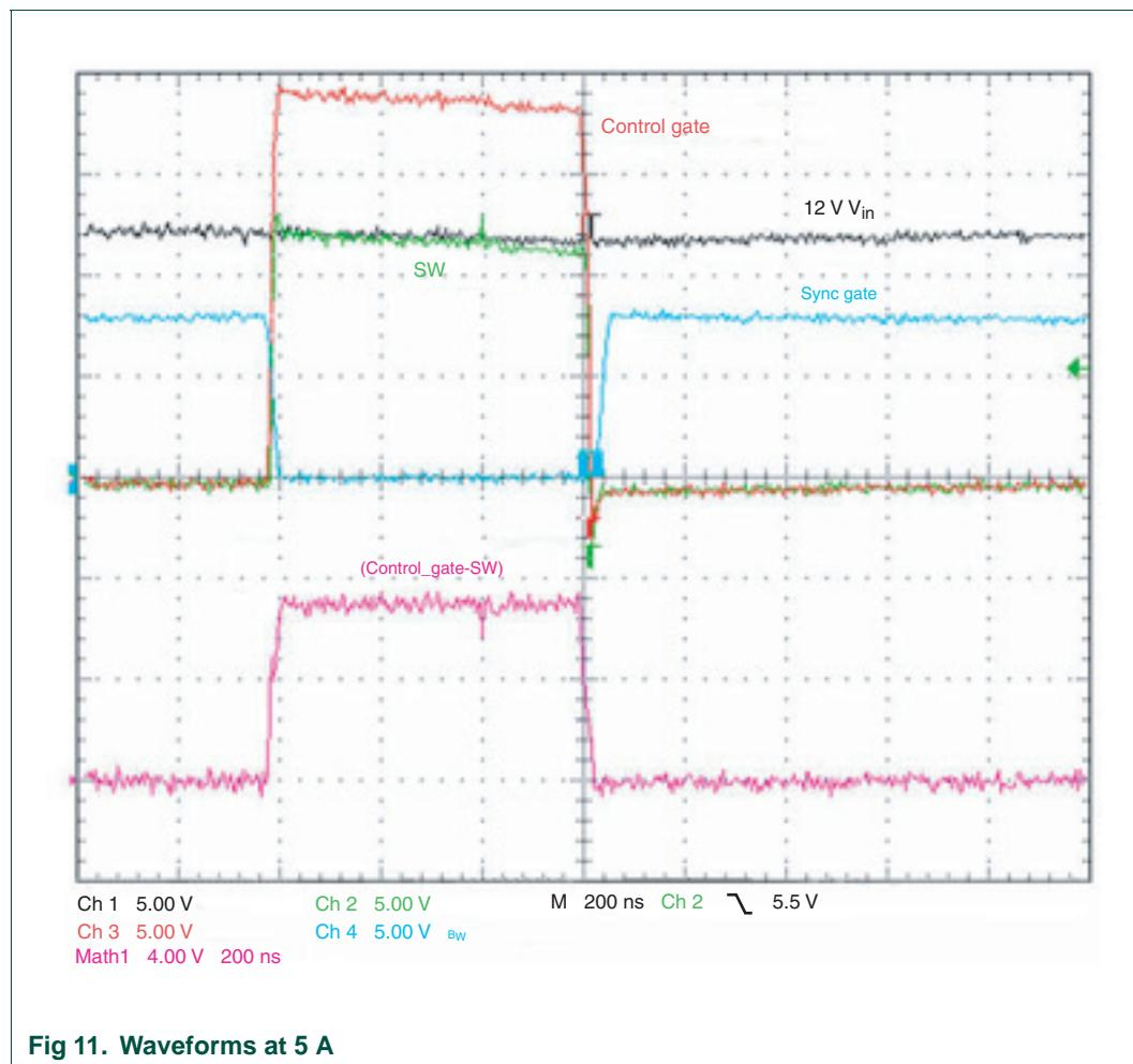
Fig 11. Waveforms at 5 A
