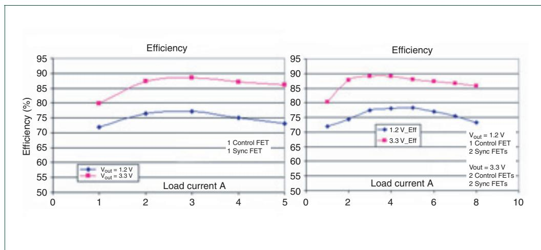
Fig 8. Efficiency sweep for 1.2 V and 3.3 V output voltages
