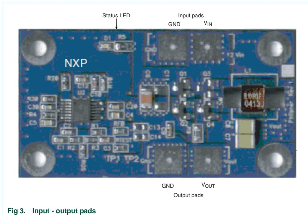
Fig 3. Input - output pads
