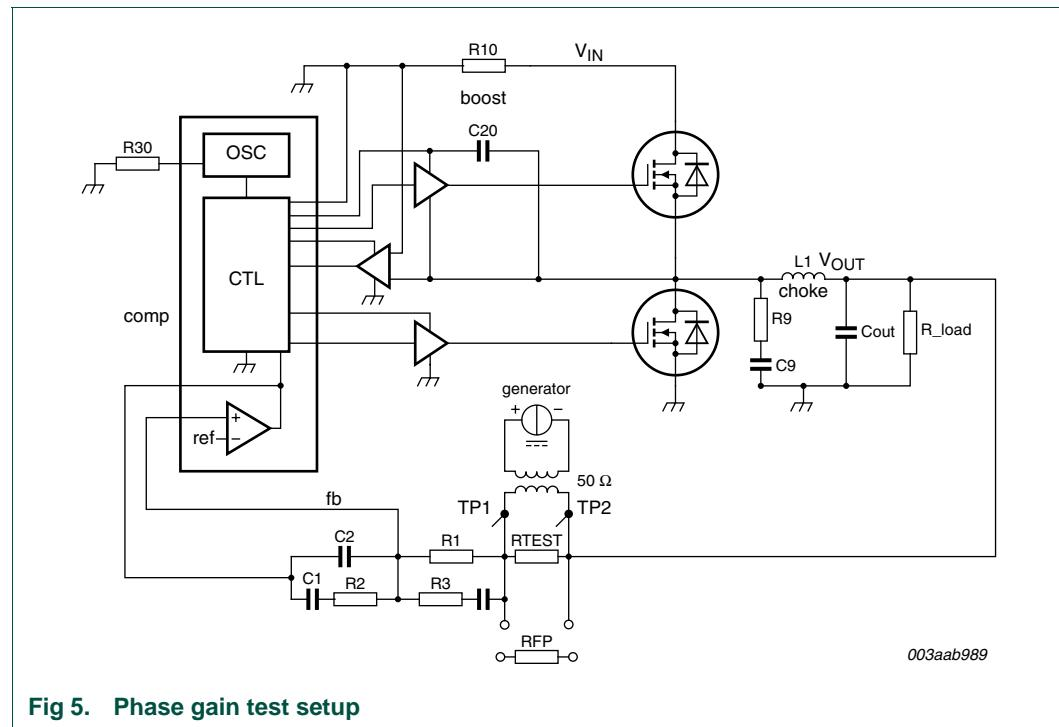
**Fig 5. Phase gain test setup**
