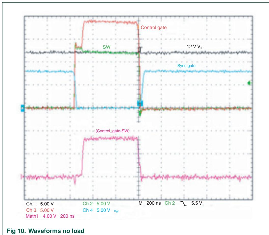
Fig 10. Waveforms no load
