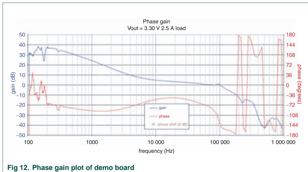
Fig 12. Phase gain plot of demo board
